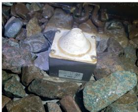
the system to the structure in just a few hours, and it had to keep on working throughout the construction programme with people and heavy machinery working just a few metres away. This system was self-powered, rugged and had no cables that would probably have been damaged by the construction activity."
