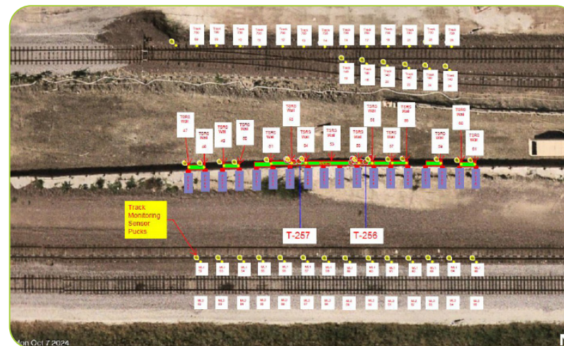
Map of sensors in the area surrounding the excavated drainage system
