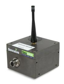
The GeoWAN Millivolt Sensor Node brings a wide variety of resistive bridge sensors into the GeoWAN system. It uses the integrated long range radio transceiver to report its measurements through Senceive's GeoWAN wireless communications network to a GeoWAN Gateway.
